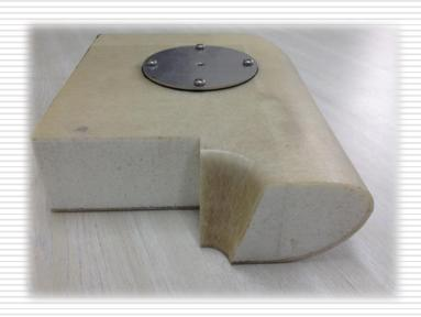
Lightweight components for solar power systems that combine LACTIF® (plant-based polylactic acid foamed beads) and polyester resin
